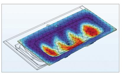
Fig. 3 Example for a 3D sinter simulation of a wash basin
