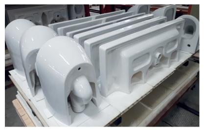
Fig. 2 Example for a kiln car loaded with six wash basins and six WC bowls
