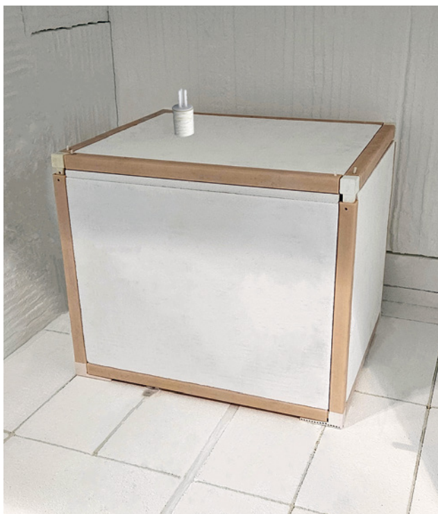
Autonomous sensor module with high temperature sensor
