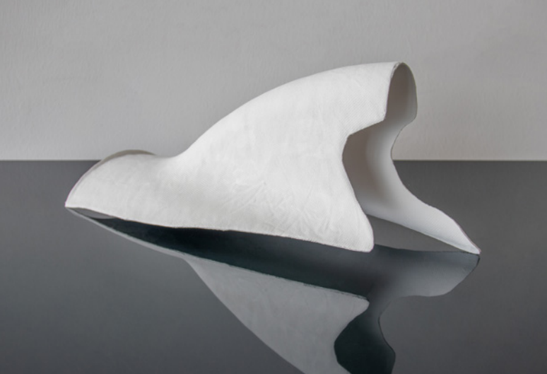
Partial segment of an exhaust mixer made of low cost CMC
