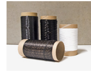
Coils with ceramic reinforcing fibres
