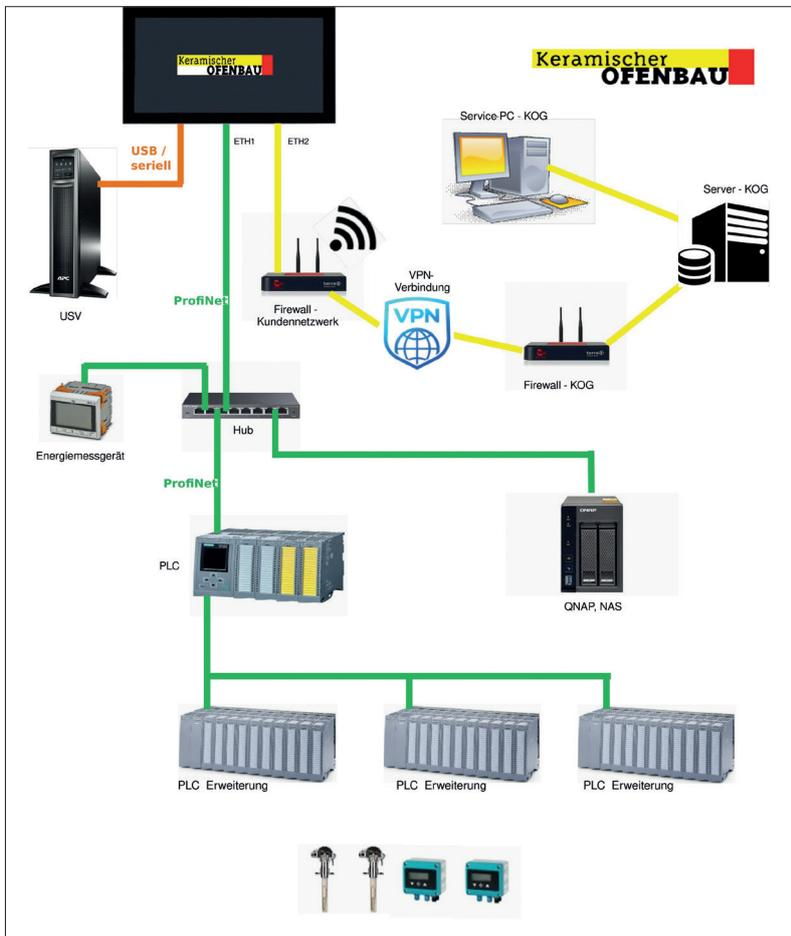
**Fig. 5** Schematic overview of data transfer between the kiln control system and the KOG servers
