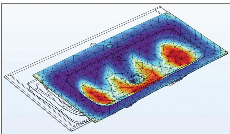
**Fig. 3** Example for a 3D sinter simulation of a wash basin
