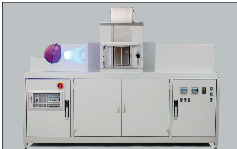
Fig. 3 New thermo-optical measuring device, TOM air , for studying debinding and sintering processes up to 1750 °C
