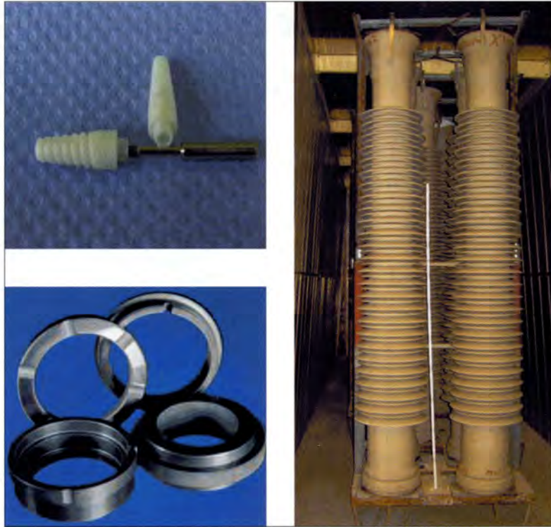
Fig. 3 Some ceramics investigated exemplarily in the project ENITEC: zirconia ceramics for dental implants (upper l.), silicon carbide seal rings (lower l.) and porcelain high voltage insulators (r.)
