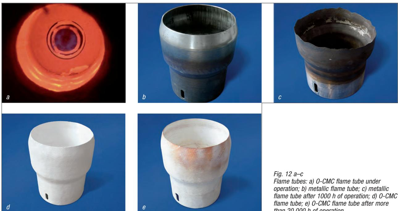
Fig. 12 a–c Flame tubes: a) O-CMC flame tube under operation; b) metallic flame tube; c) metallic flame tube after 1000 h of operation; d) O-CMC flame tube; e) O-CMC flame tube after more than 20 000 h of operation
