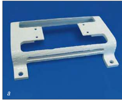
Fig. 7 a–b O-CMC parts machined with diamond tools
