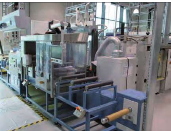
Fig. 6 Fabrication of prepreps at the lab
