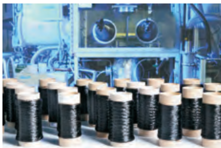
Fig. 4 Realization of melt-spinning process and produced ceramic high-tech fibers
