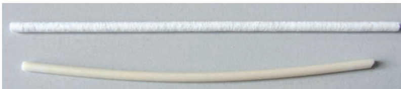
Fig. 6 Solid rods (diameter 3,3 mm) made out of RAMUL-HT (top) and a benchmark material (bottom) after 5 kiln cycles at a dwell temperature of 1600 °C
