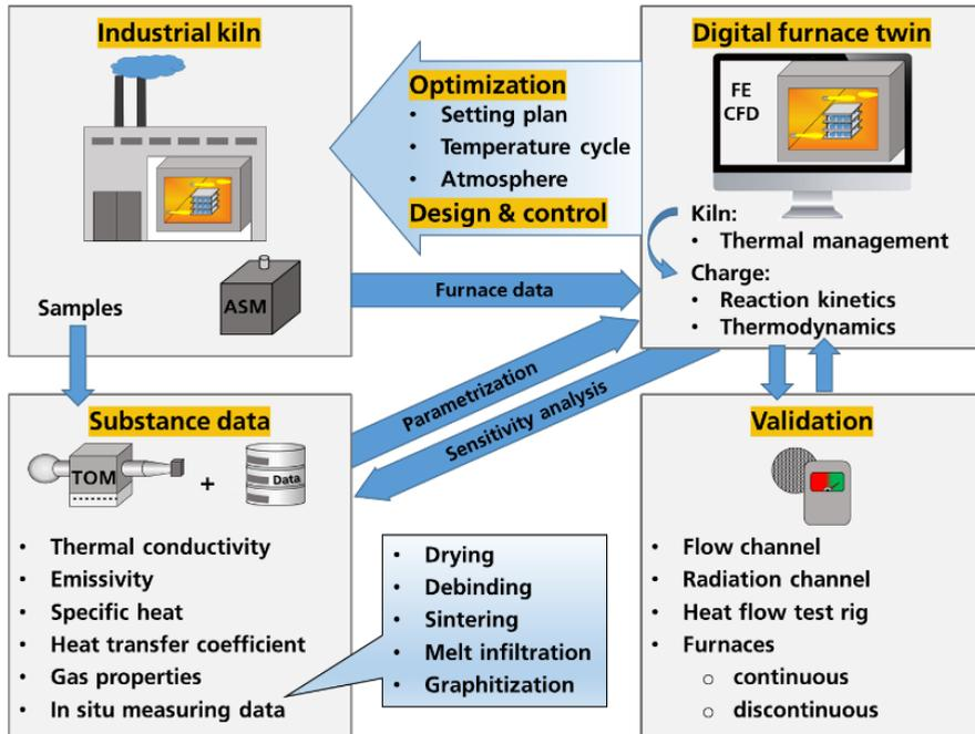
Fig. 1.1 Interaction of methods for a high-quality digital furnace twin
