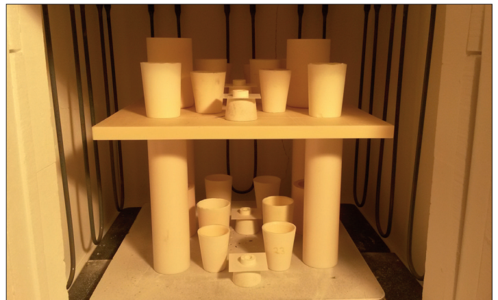
Fig. 6 Set-up of a small batch furnace for alumina sintering
