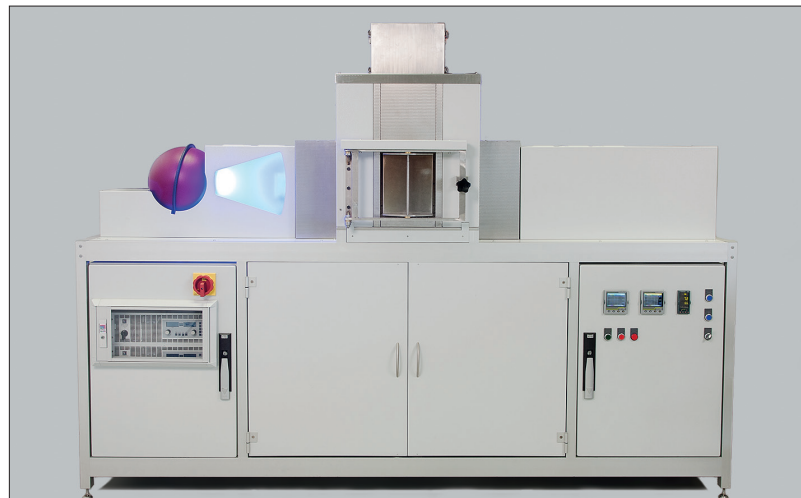
Fig. 3 New thermo-optical measuring device, TOM air , for studying debinding and sintering processes up to 1750 °C
