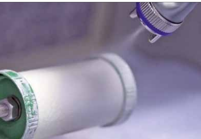
Fig. 2 Application of the sealing material onto a plasma-sprayed alumina tube via spraying
