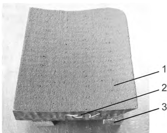
Fig. 5. Charged CARBOTEX® sample (thickness: 20 mm, length: 80 mm, width: 80 mm). – 1: environmental barrier coating made of silicon slurry, 2: CARBOTEX® substrate, 3: graphite bars as support auxiliaries.
