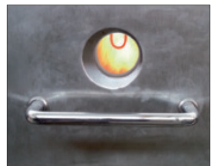
Fig. 9 Inspection glasses of transparent spinel ceramics for high temperature application (Source: CeramTec-ETEC GmbH)
