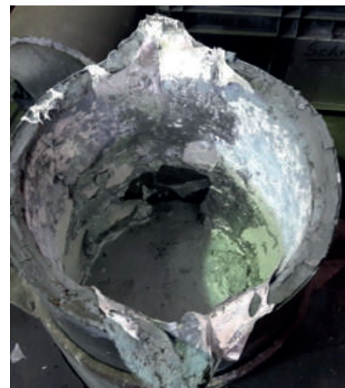
Fig. 10 Used casting crucible with ceramic fabric lining (Source: Metallgießerei Chemnitz)
