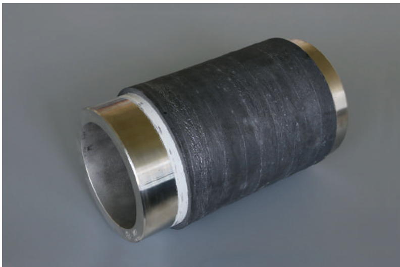
Fig. 11 CMC reinforcement for power plant steel pipes (Source: Fraunhofer-Centre HTL)
