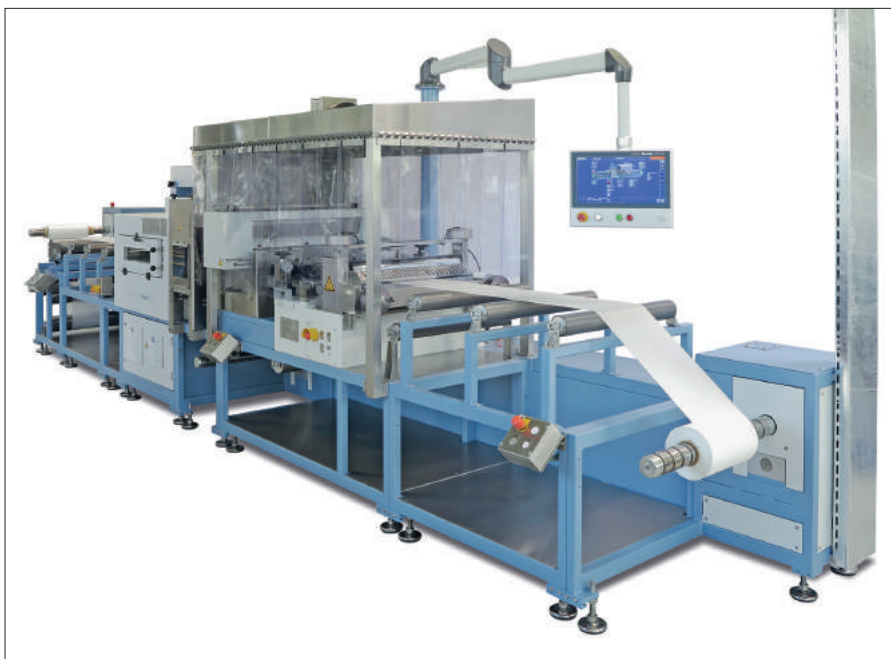
Fig. 5 Fabric prepreg plant at Fraunhofer-Centre HTL
