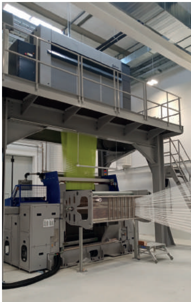
Fig. 3 Double rapier weaving machine with single-thread operation (Source: Fraunhofer-Centre HTL)
