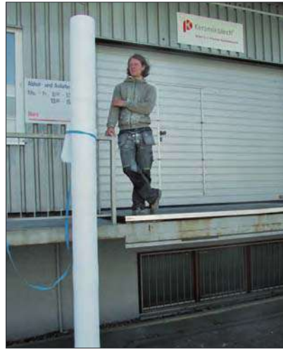
Fig. 16 Large-sized O-CMC thermal protective tube built with modular design
