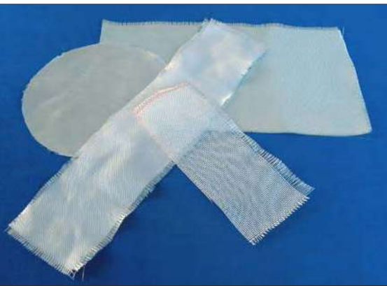
Fig. 1 Oxide ceramic fibres as woven fabric
