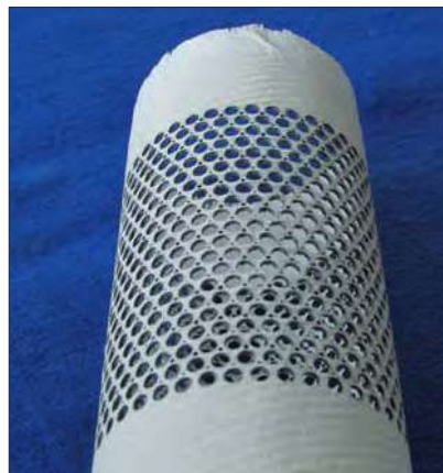
Fig. 9 Example of a tube with a hole pattern done by laser machining
