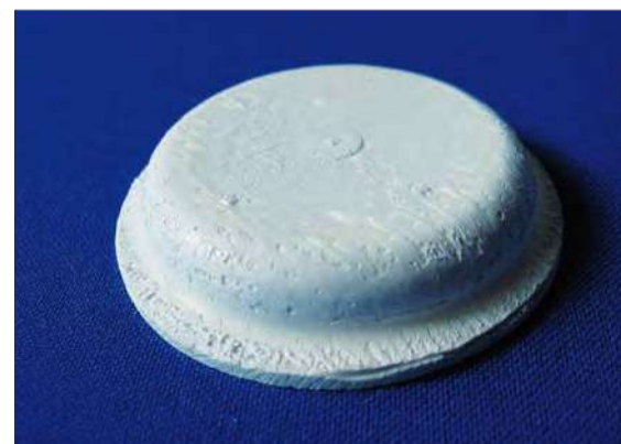
Fig. 4 Green body of O-CMC material after pressing in mould
