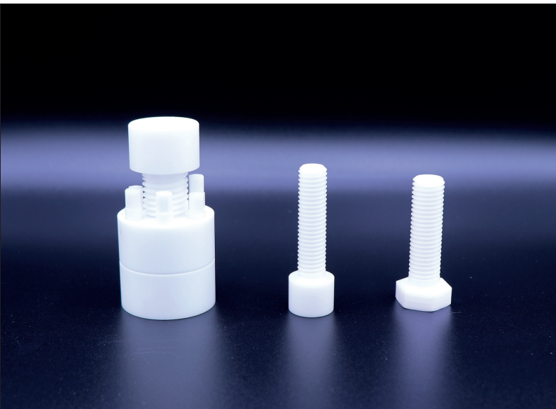
Fig. 1 ZrO 2 superbolt demonstrator and ZrO 2 screws (thread size M10) with standard metric thread geometry and with suitable-to-ceramic geometry (f. l. t. r.)
