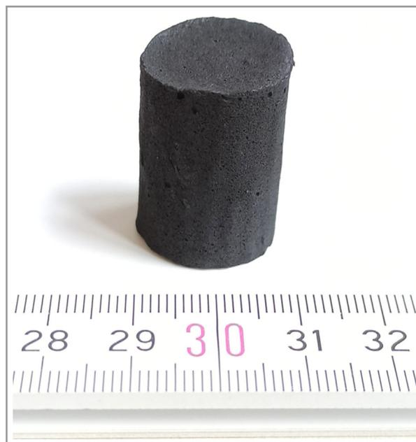
Figure 2. Image of a carbon foam.
