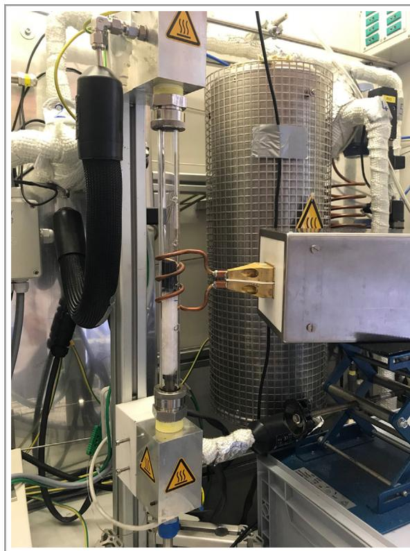
**Figure 1.** Experimental setup of reactor for catalytic testing in combination with induction heating. A carbon foam is placed inside of the inductor.
