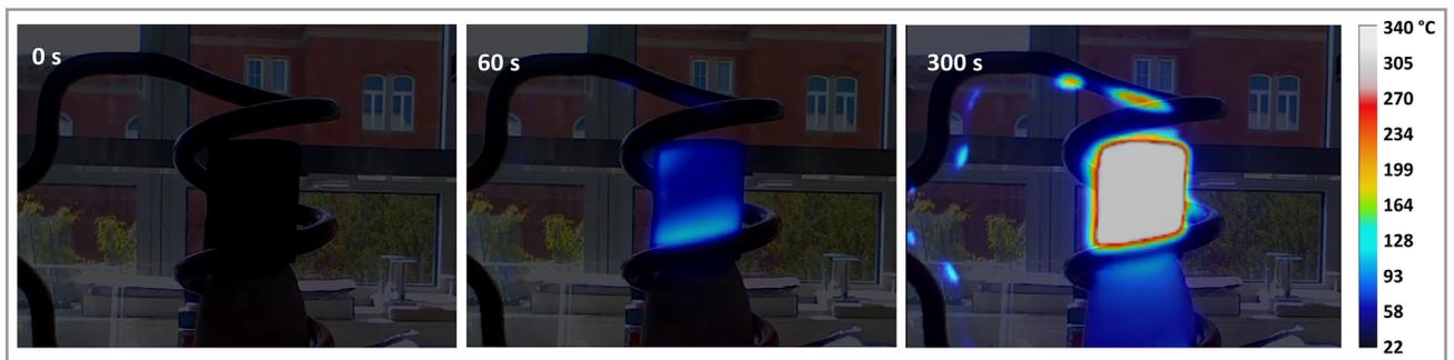
**Figure 6.** Thermal camera images of induction heating process of the carbon foam CFF-50M.
