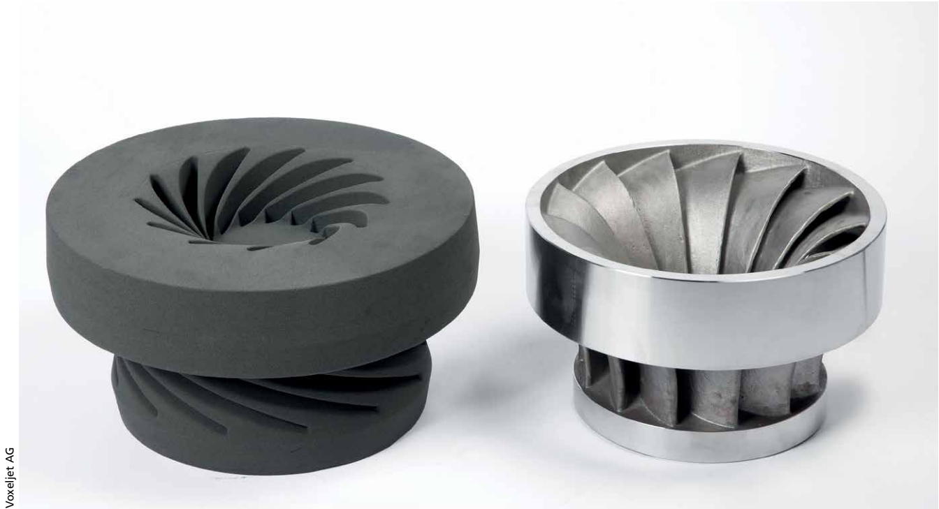
3-D-printed sand core (left) and final casted part (right).
