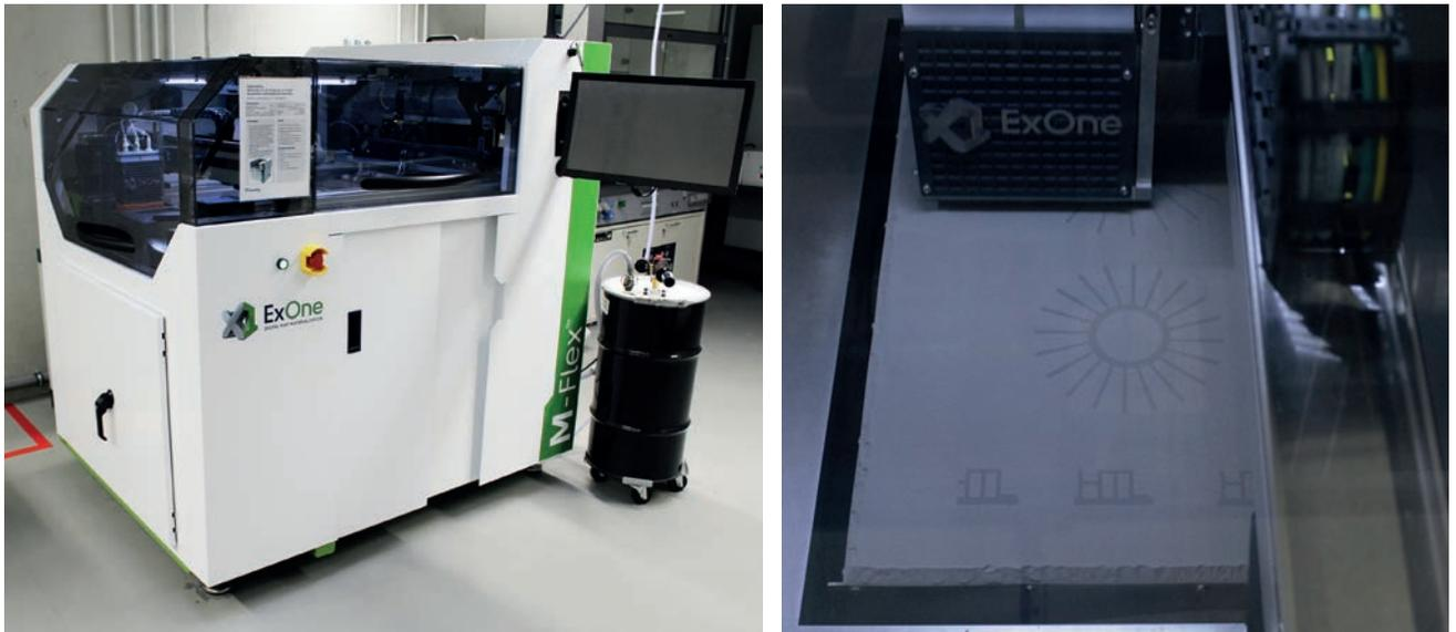
**Fig. 4** Binder Jetting printer (M-Flex) (l.), and a view on its print-head and powder-bed during operation (r.)
