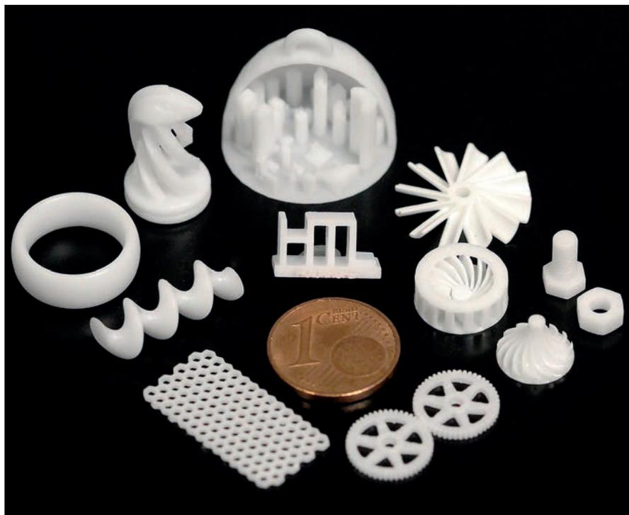
**Fig. 2** Examples of high purity alumina parts manufactured via the stereolithography process
